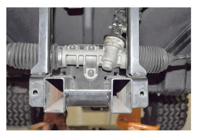
${\bf 1. Remove\ front\ cover.\ Then\ remove\ OEM\ control\ arms\ and\ spindles\ from\ cart.\ Save\ hardware\ for\ use\ in\ later\ steps.}$
