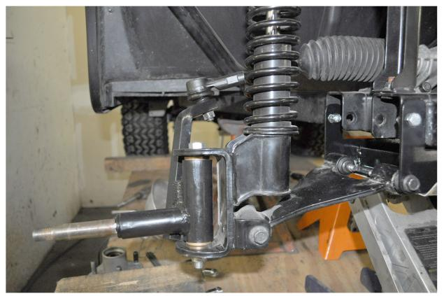
5. Attach new spindles to control arms using included 1/2" x 6" bolts, nylocs and SAE washers. Then attach tie rods to steering arms on spindles using OEM hardware. Tighten hardware and repeat for opposite side.6. Re-install OEM hubs on new spindles.
