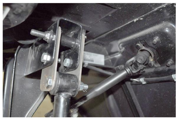
3. Unbolt shock from stock location and re-attach with shock extension plates. Attach plate at top with OEM bolt and nyloc with spacer in-between. Attach mid-section with two  $3/8'' \times 1''$  bolts and nylocs. Attach shock to plate with  $3/8'' \times 2 1/2''$  bolt with nyloc. Tighten hardware. Repeat for opposite side.
