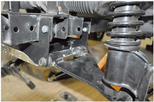
4. Bolt control arms to bottom of the carrier using OEM bolts and nylocs. Tighten hardware.
