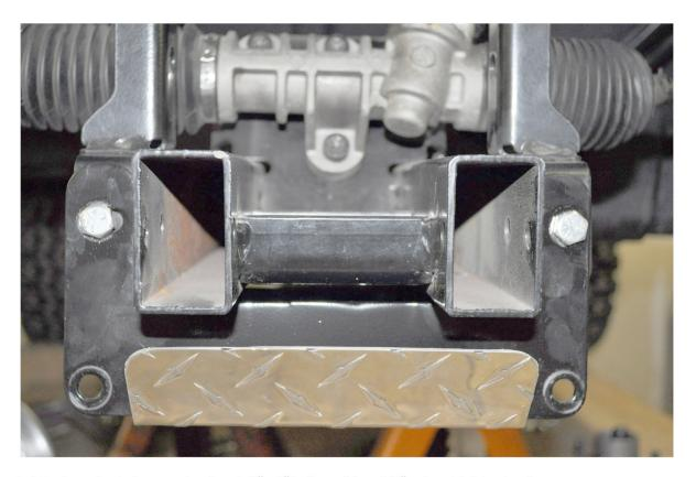
2. Attach carrier to frame using four 3/8" x 1" bolts and four 3/8" nylocs. Tighten hardware.
